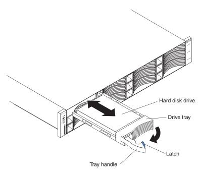
Figure 46. Removing a drive
